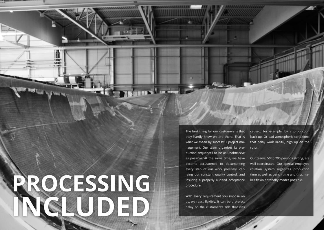
Production of rotor blade components; pre-finishing and finishing of the rotor blades themselves
